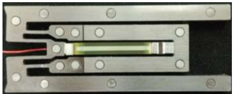
ViVa 3mm Actuator configured as single stage with two toggle arms.
